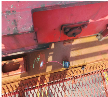
Fig. 5. Stress tested point 1 and sensor
