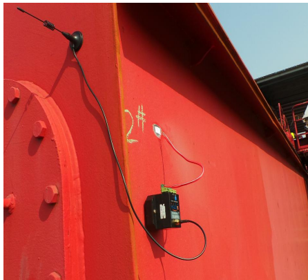
Fig. 6. Stress tested point 2 and sensor
